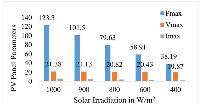
**Fig. 7. Different Solar PV Parameters at 35°C**
