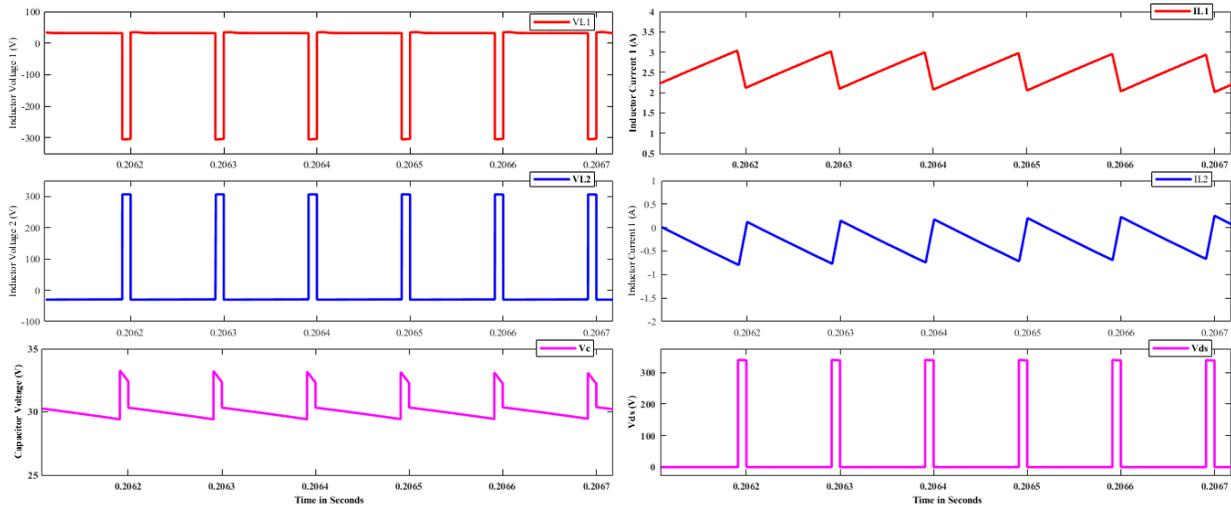
**Fig. 11. Converter Waveforms for Various Irradiation with Constant Load; (a) Inductor ( $L_1$ ) Voltage in Volt. & Inductor ( $L_1$ ) Current in Amp., (b) Inductor ( $L_2$ ) Voltage in Volt. & Inductor ( $L_2$ ) Current in Amp., (c) Voltage across the Coupling Capacitor in Volt., (d) Switch Voltage in Volt**
