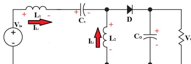
**Fig. 4. Current Flow when  $Q_1$  in OFF State**
