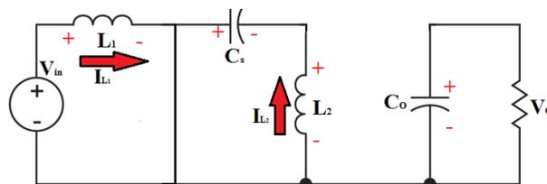
**Fig. 5. Current Flow when  $Q_1$  in OFF State**
