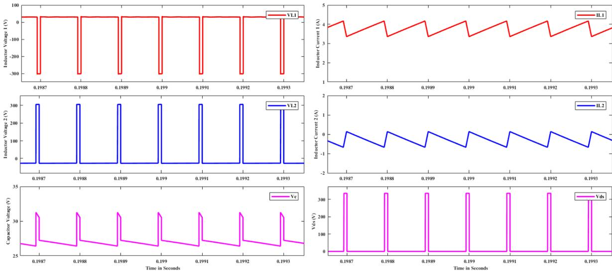
**Fig. 9. Converter Waveforms for Various Irradiation with Constant Load; (a) Inductor ( $L_1$ ) Voltage in Volt. & Inductor ( $L_1$ ) Current in Amp., (b) Inductor ( $L_2$ ) Voltage in Volt. & Inductor ( $L_2$ ) Current in Amp., (c) Voltage across the Coupling Capacitor in Volt., (d) Switch Voltage in Volt**
