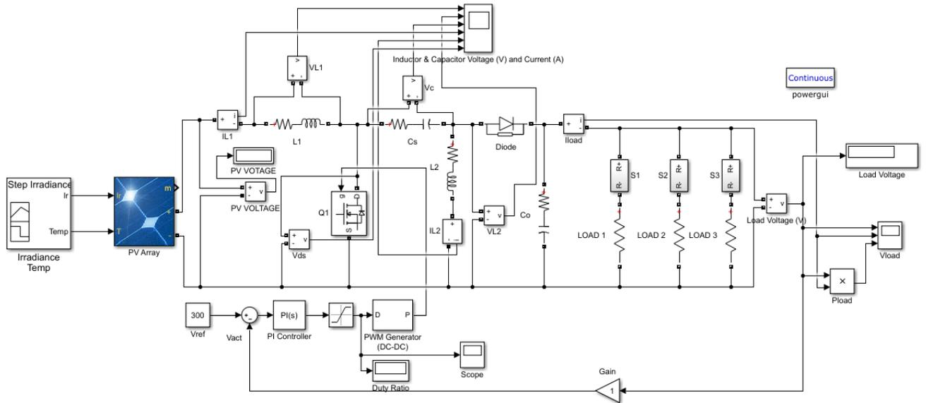
**Fig. 6. Simulation Model of the SEPIC Converter**
