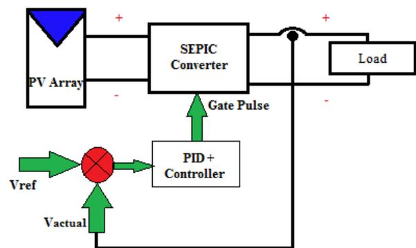
Fig. 2. Block Diagram for the Closed Loop Control
