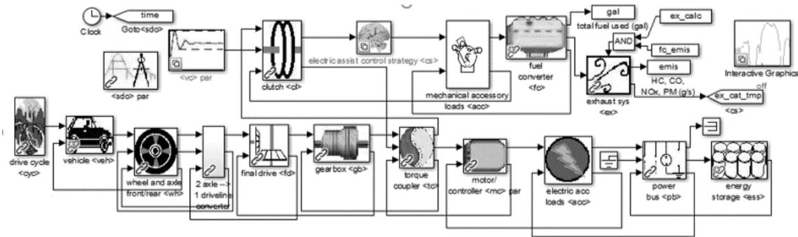
Fig. 8. Simulation vehicle block diagram
