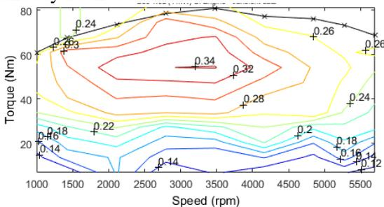
Fig. 2. Engine fuel consumption map
