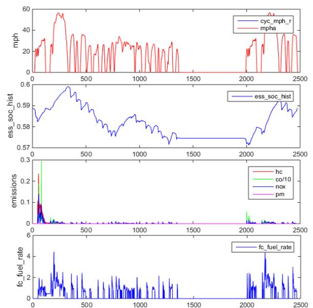
Fig. 9. BABC Fuel usage, emission and SOC plot
