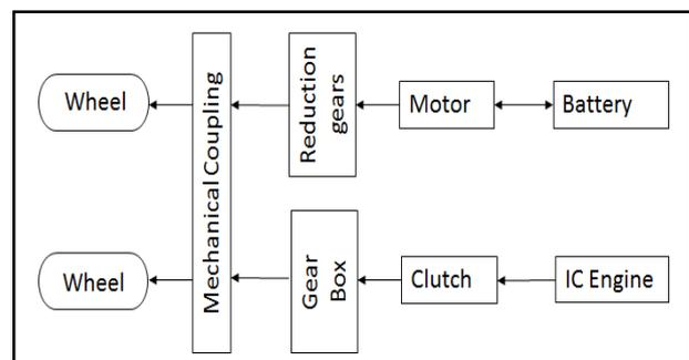
Fig. 1. Parallel HEV Block Diagram
