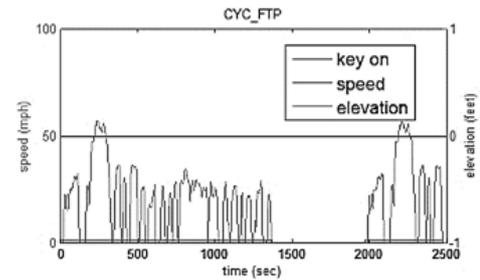
Fig. 5. FTP driving cycle
