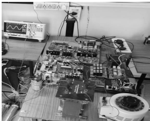
Figure 17. Hardware implementation of 15level MLI with single input triple output DC-DC boost converter
