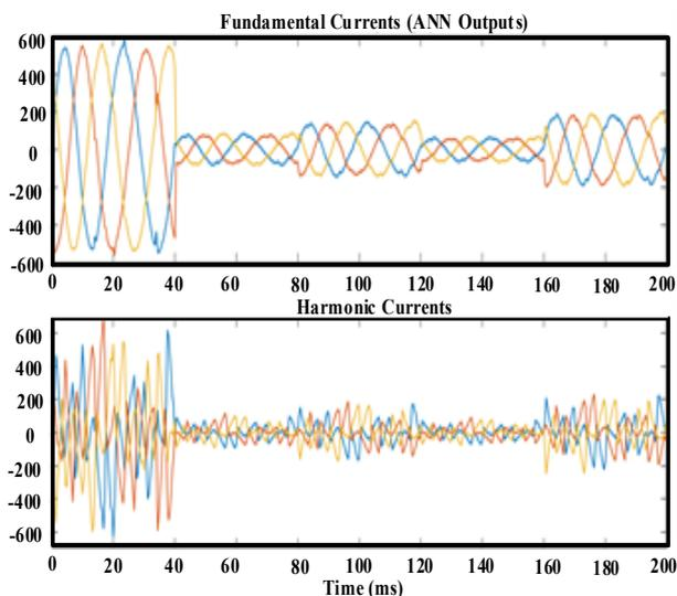
Fig. 8. Waveforms of RBF network outputs (upper) and harmonic currents (lower)
