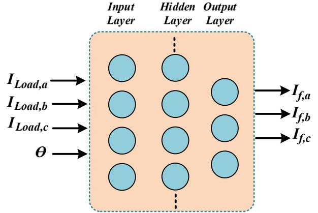
Fig. 4. The structure of RBF network
