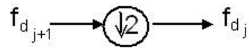
Figure 2.24: Relation between the filters corresponding to two consecutive levels of UDWT reconstruction
