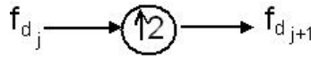
Figure 2.22: Relation between the filters corresponding to two consecutive levels of UDWT decomposition
