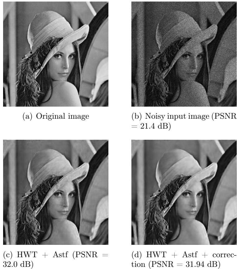
Figure 5.16: HWT - Adaptive soft-thresholding denoising results applied on Lena affected by multiplicative noise
