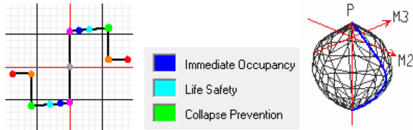
Figure 5.9: a) Moment – rotation relation based on FEMA procedure; b) P-M-M surface interaction
