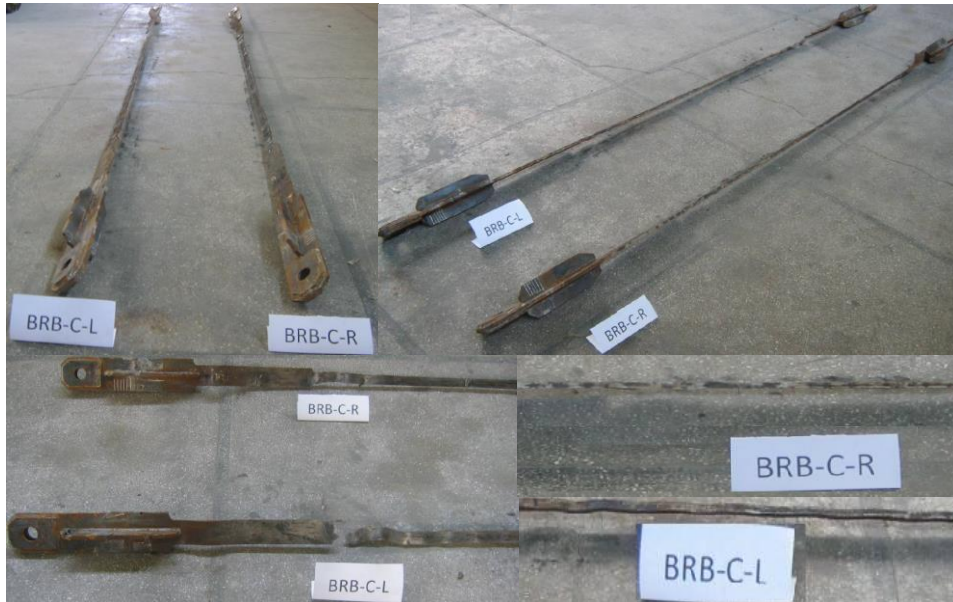
Figure 6.34 BRB steel core plates during cyclic test
