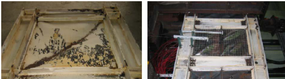
Figure 2.30 Typical photographs showing specimen at the ultimate stage [23]
