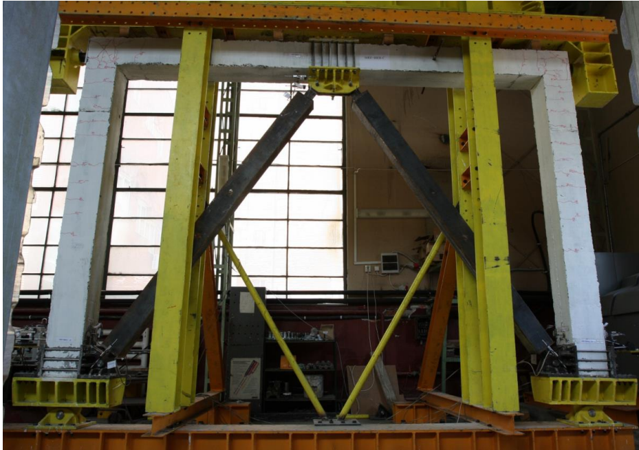
Figure 6.28 MRF + BRB under cyclic load
