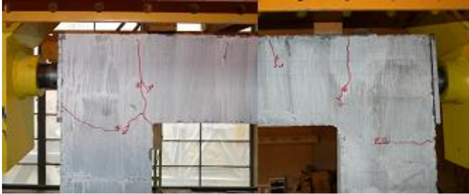
Figure 6.25 RC frame under cyclic load – development of bending cracks
