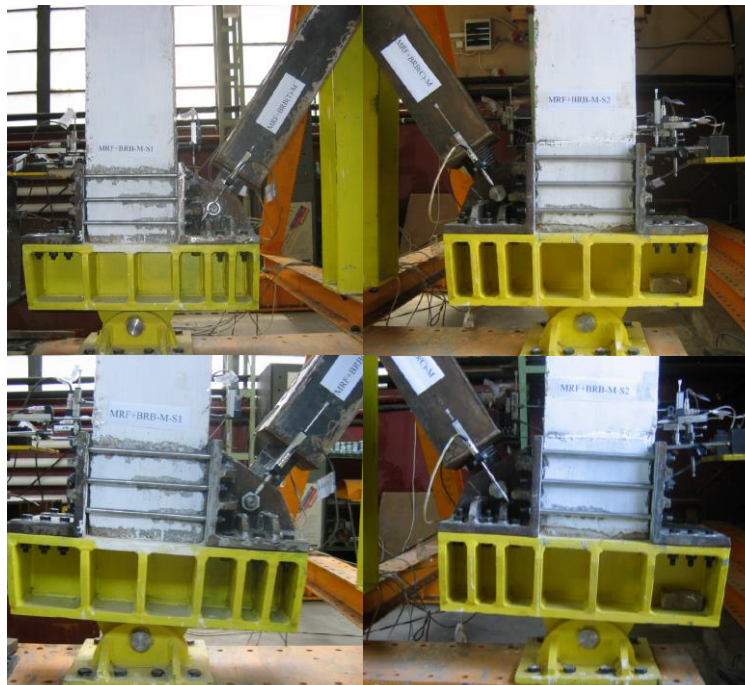
Figure 6.35 BRB to column connection after cyclic test
