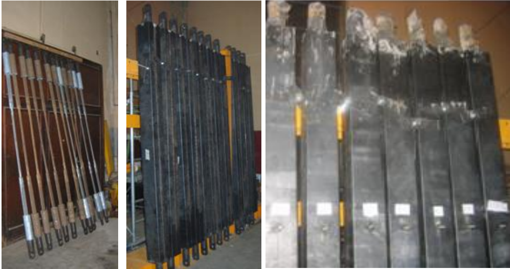
Figure 4.6 Manufacturing of BRB elements: wrapped BRB elements; centering and fixing inside the tubes; pouring the concrete in vertical position
