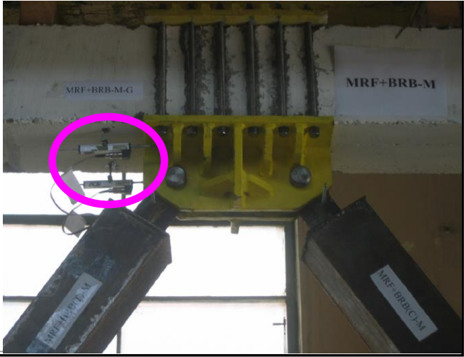
Figure 6.17 Measurement devices distribution: Horizontal on the RC beam
