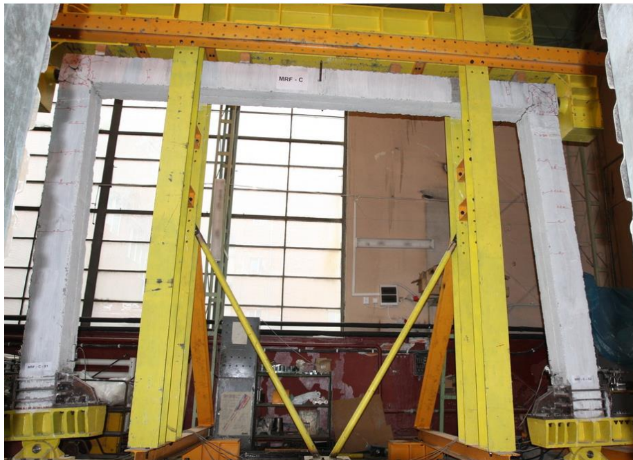
Figure 6.24 RC frame under cyclic load
