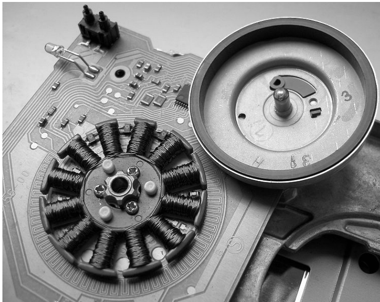
Fig. 1.24. Pancake PM brushless motor with 12 concentrated stator coils and outer rotor with ring-shaped PM. The stator is integrated with control electronics.
