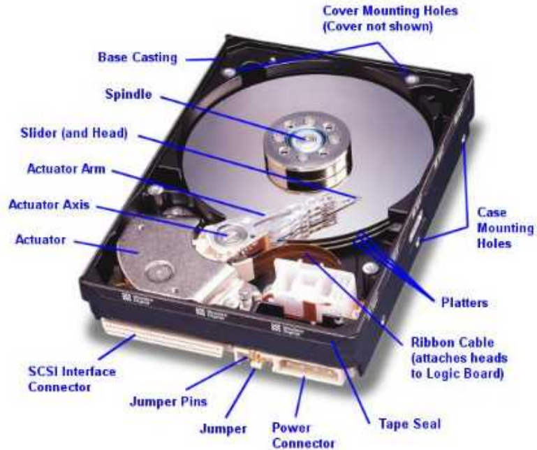
Fig. 1.23. An example of hard disk drive. The disk drive spindle motors are brushless DC motor with outer rotors designs.
