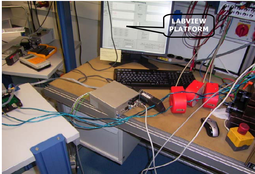
Fig. 3.39. The setup used to measure the back-EMF.
