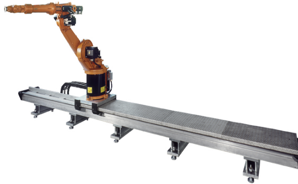
Figure 4.2: Industrial robot on linear track
