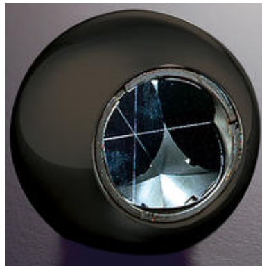
Figure 6.2: Corner Cube Reflector
