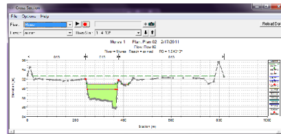
Fig. 9 Determining the level at Nadlac hydrometric station
