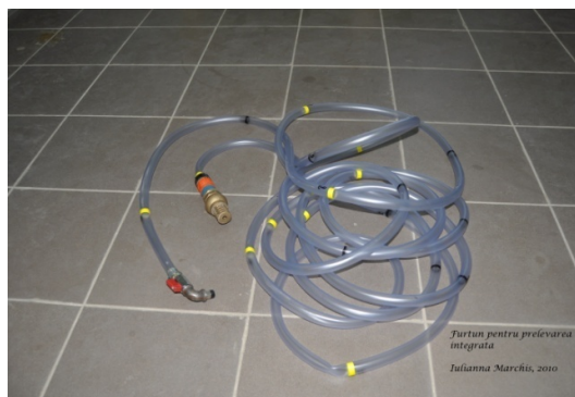
Fig. 2. Integrated water sampling hose
