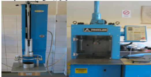
a) Marshall hammer b) Gyratory compactor Figure 3. Equipment used in manufacturing the samples
