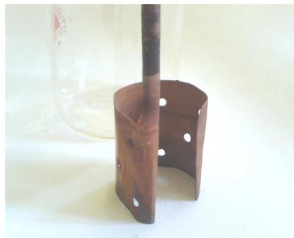
Figure 3. Copper anode
