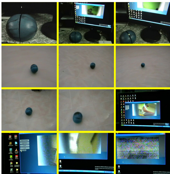
Fig. 14. Snapshots of the spy ball while moving in speed, rotating, while still and when taking an image from the camera along with video feed display by the software
