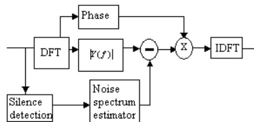
Fig.1. Block diagram of a spectral subtraction system
