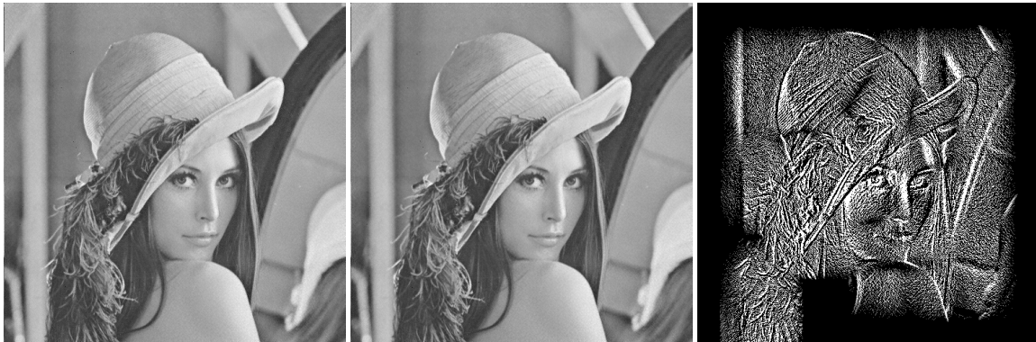
Fig. 7: (left) Watermarked image for the HWT based method, having a PSNR=35.60 dB and a weighted PSNR=52 dB compared to the original Lena, (middle) Distorted watermarked with the LPCD attack N=5 and L=6 with PSNR=28.16 dB, weighted PSNR=37.87 dB, (right) Difference between the two images, magnified 100 times
