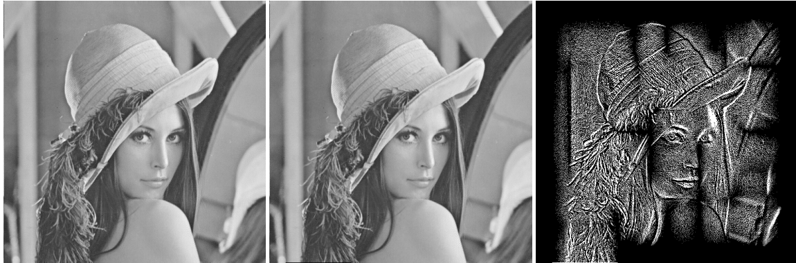
Fig. 6: (left) Watermarked image for Barni's method [13], having a PSNR=36.39 dB and a weighted PSNR=33.20 dB compared to the original Lena, (middle) Distorted watermarked with the LPCD attack N=5 and L=6 with PSNR=30.68 dB, weighted PSNR=30.82 dB, (right) Difference between the two images, magnified 100 times
