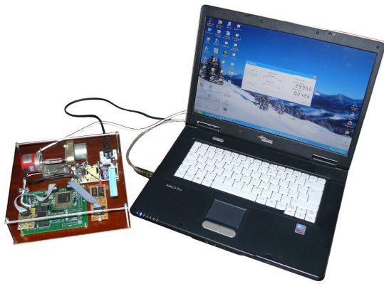
Fig. 6. Overview of experimental measuring system with rotary incremental encoder
