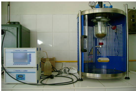
Figure 1. Experimental installation for gold lixiviation
