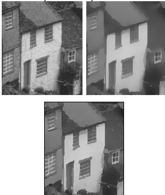
Fig.7 Removal of blocking artifacts using the proposed fusion/diffusion approach. From top to bottom and left to right: original image, Perona Malik filtered image, result using the proposed approach
