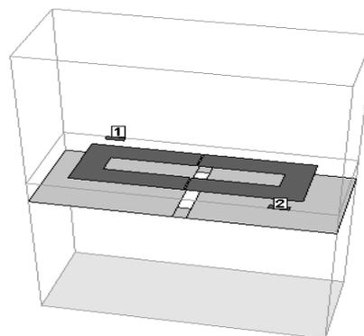
Fig. 1. Geometry of the investigated microstrip DGS
