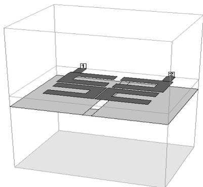
Fig. 11. 3D view of the DG band-pass filter
