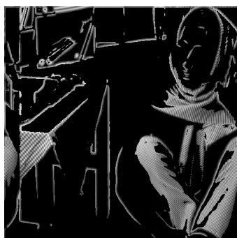
Fig. 2. The class corresponding to the interval I_6 , contains the contours and the larger textures.
