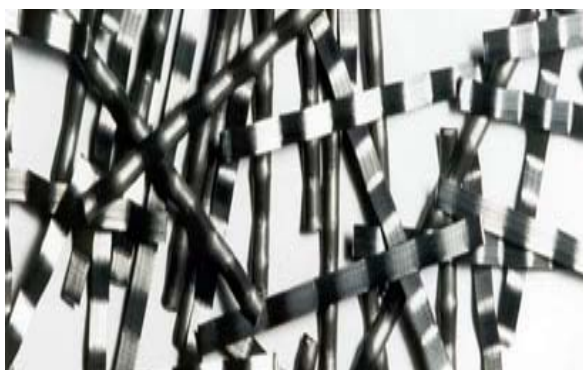
Fig. 5. Fibre metalice rectangulare (plate)
