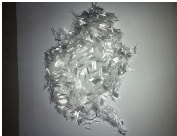
Figura 35. Fibre polimerice monofilament RoWhite 12 mm[28]
