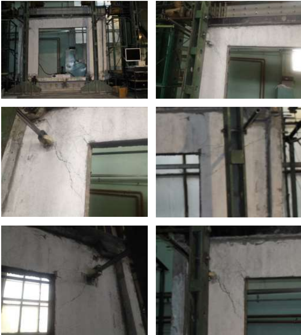
Figure 4-5 – Failure details of PRCWP 18-L3-E3-T
