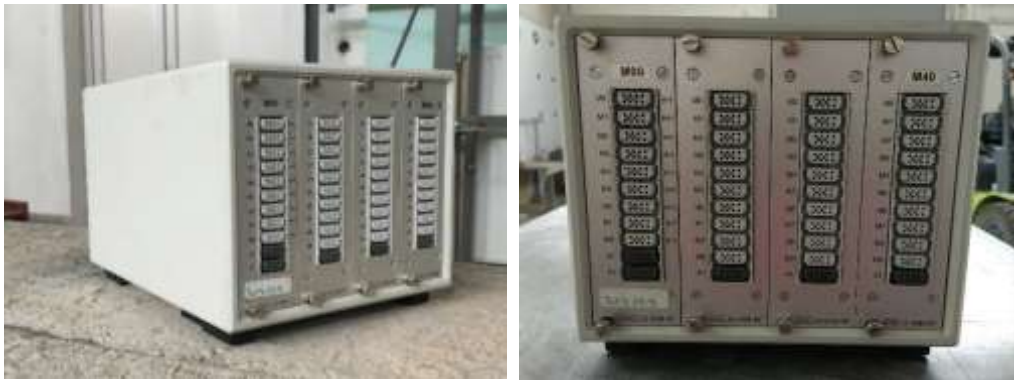
Figure 3-28 – Data acquisition system
