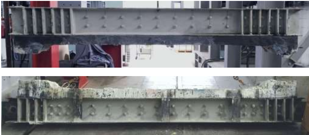
Figure 3-21 – Casted loading beams
