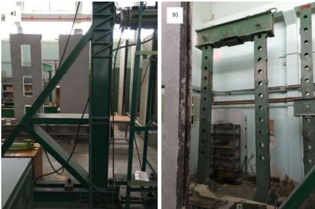
Figure 3-24 - Lateral and vertical reaction frames
