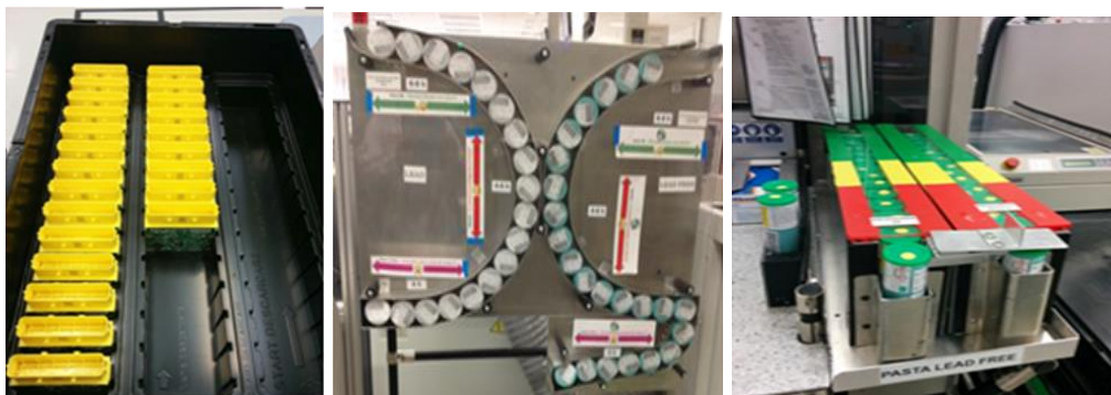
Figure 2.38. Adjustable separators (left), solder paste storage and quick identification: before (middle) and after (right)
