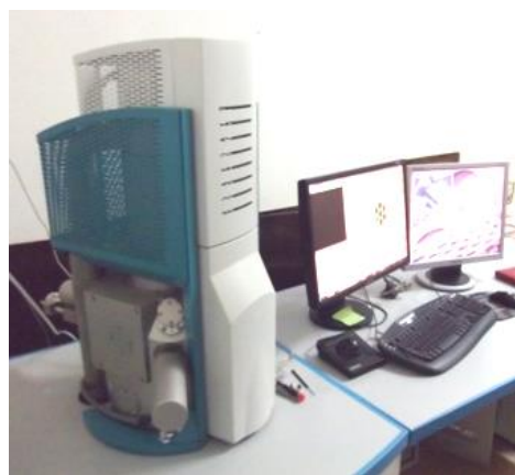
Fig.2.10. Microscopul electronic cu baleiaj TESCAN VEGA 3 LMU Bruker EDX Quantax
