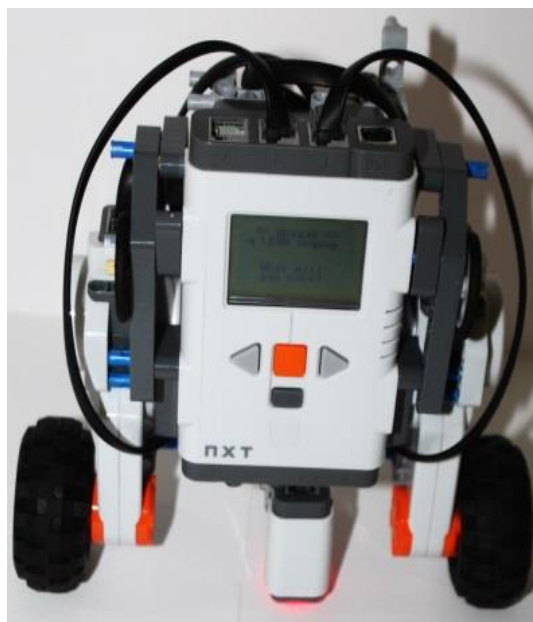
Figura 5.1 Robot mobil humanoid – demonstrator mecatronic echipat cu senzor optic
