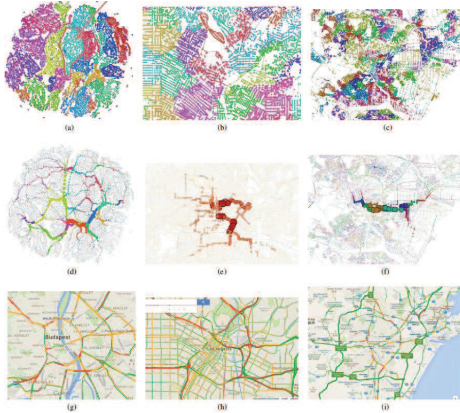
Figure 32. Case study data sets regarding traffic hotspots in three cities taken into consideration: Budapest, Downtown Los Angeles and Sendai; Subfigures (a), (b), (c) show the identified communities after applying the first step in SIGS; Subfigures (d), (e), (f) display the identified “backbone” of the city, the nodes with high betweenness have larger size; Subfigures (g), (h), (i) represent data captures from Google Traffic Layer showing traffic conditions in the areas of interest
