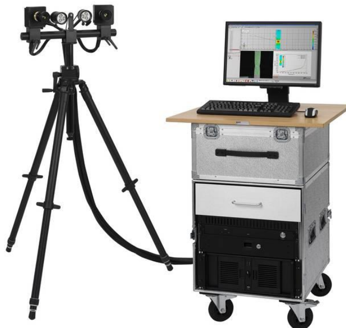
Figure 3—21 DIC hardware and software.
