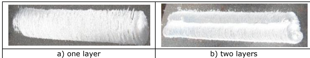
Figure 2—8 Deposition of EN AW 7050, using tool having diameter \Phi 12 mm
