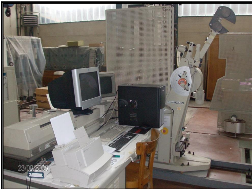
Figure 3—6 The instrumented Charpy pendulum SCHNECK TREBEL 300 J
