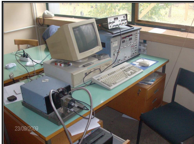
Figure 3—17 High-frequency pulsator FRACTOMAT
