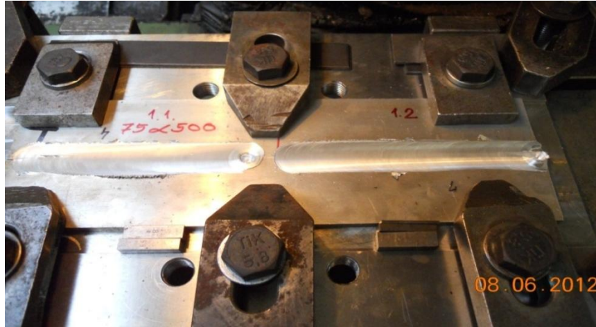
Figure 3—3 Clamps of work piece to machine FSW.
