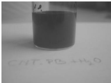
Fig. 33: Plasma treated CNT dispersed in H 2 O
