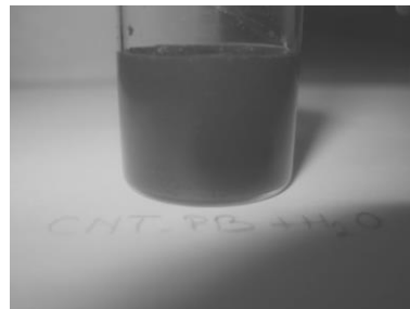
Fig. 34: Plasma treated CNT dispersed in H 2 O after 60 minutes
