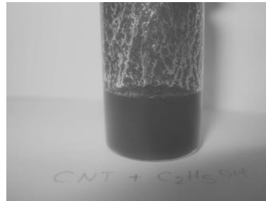
Fig. 32: CNT dispersion in C 2 H 5 OH (w/o previous plasma treatment)
