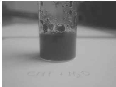
Fig. 31: CNT dispersion in H 2 O (w/o previous plasma treatment)
