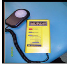
Figure 8-b: Measurement of illumination E with luxmeter on the dental seat unit.
