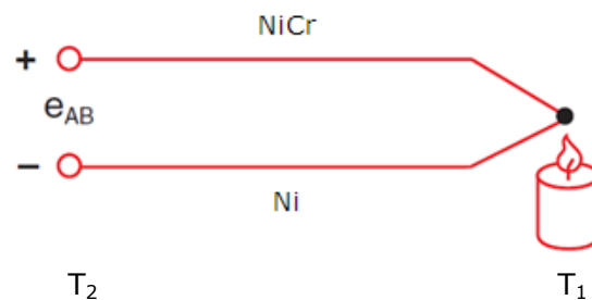
Figure 3.5: Open voltage circuit; e_{AB} = Seebeck voltage
