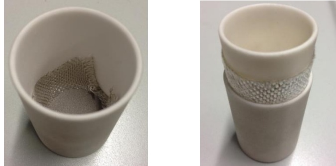
Figure 4.4: Ceramic crucible, refractory-lined with a glass fiber mat (left) and sealed ceramic crucible with the powder (right)
