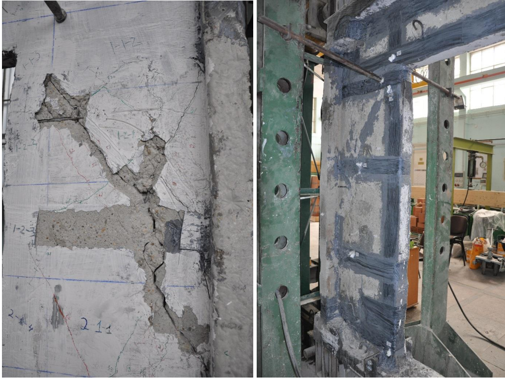
Figure 3.2 - Failure details of the PRCWP (8-E3-T/R) specimen [109, 112, 115]
