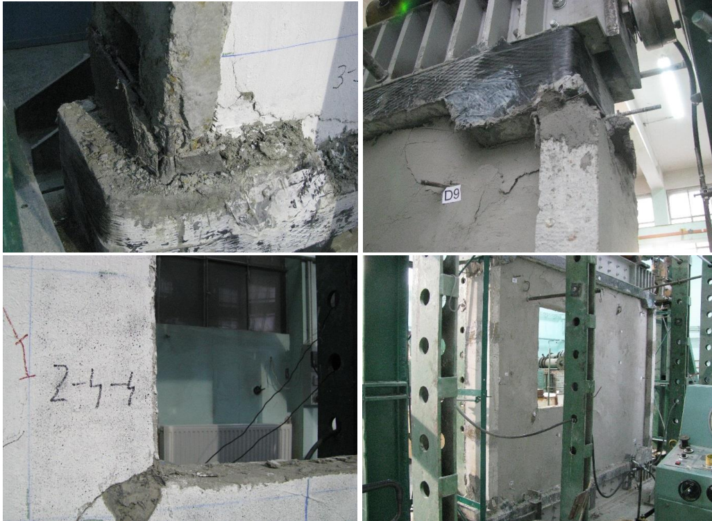
Figure 3.5 - Failure details of the PRCWP (11-L1-T/R) specimen [109, 113-114]
