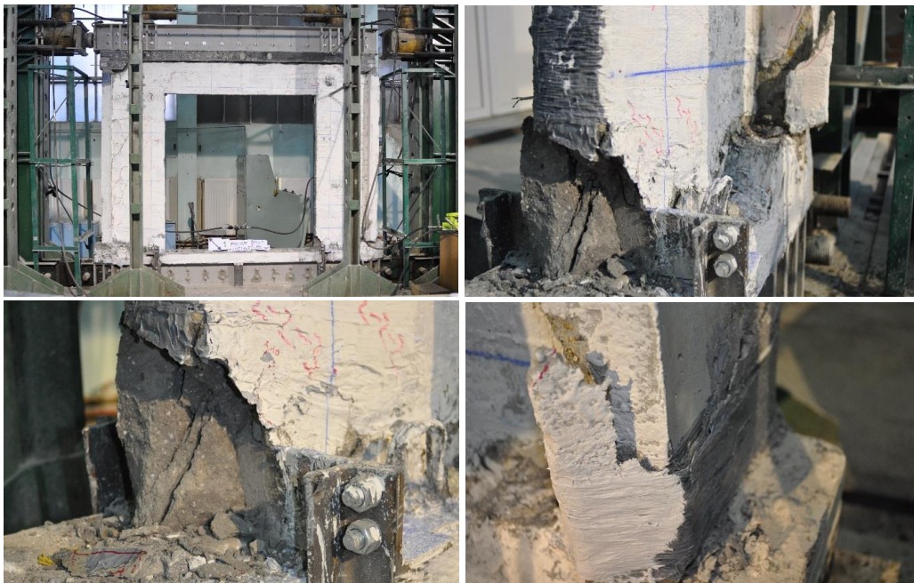
Figure 3.2 - Failure details of the PRCWP (8-E3-T/R) specimen [109, 112, 115]
