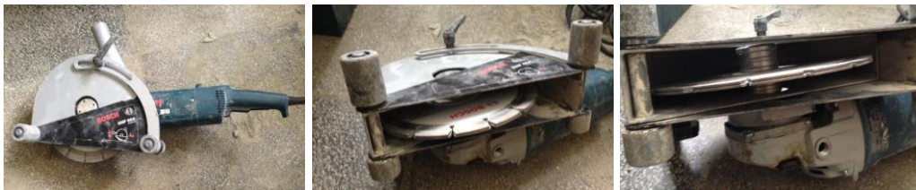
Figure 2.32 – Double disc grinder used for the NSM channel cut
