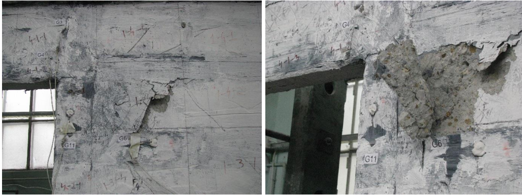
Figure 3.1 - Failure details of the PRCWP (7-E1-T/R) specimen [109-110, 112, 115]
