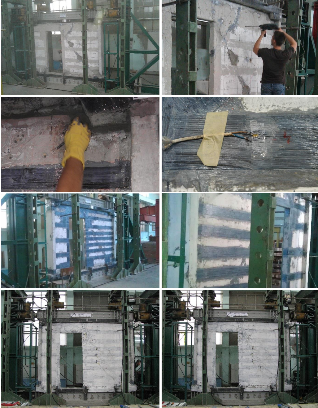
Figure 2.27 – FRP strengthening details
