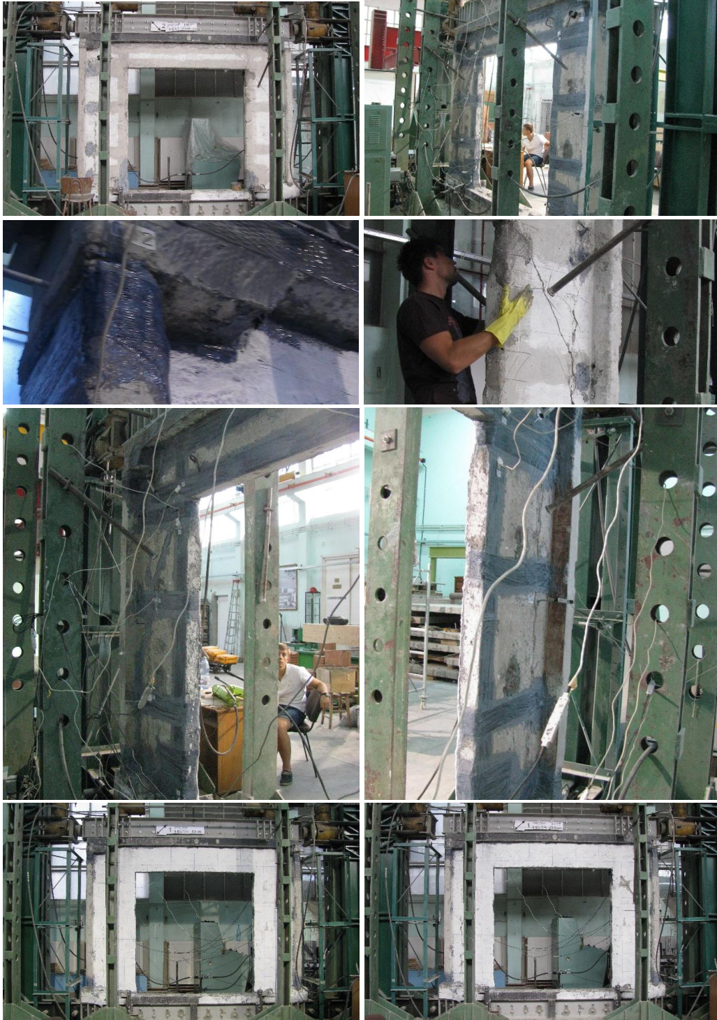
Figure 2.29 – FRP strengthening details
