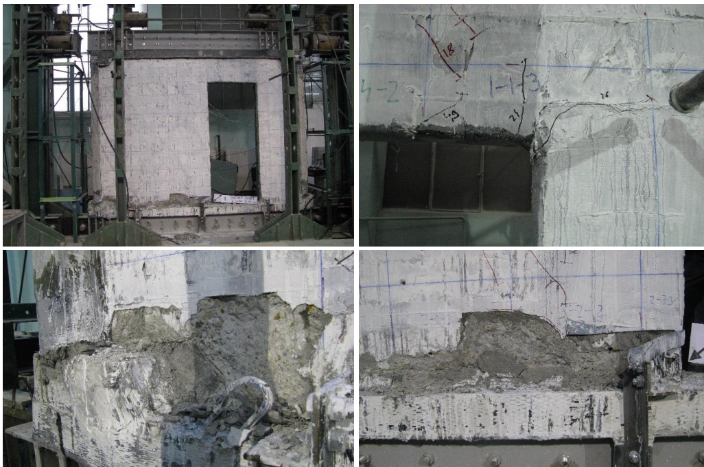
Figure 3.5 - Failure details of the PRCWP (11-L1-T/R) specimen [109, 113-114]
