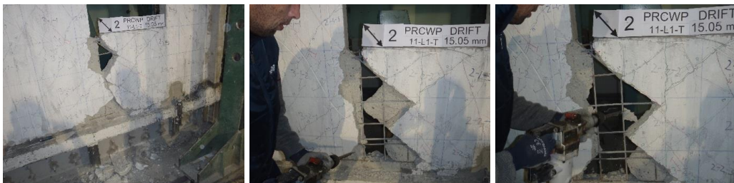
Figure 2.38 – FRP strengthening layout for PRCWP (11-L1-T/R)
