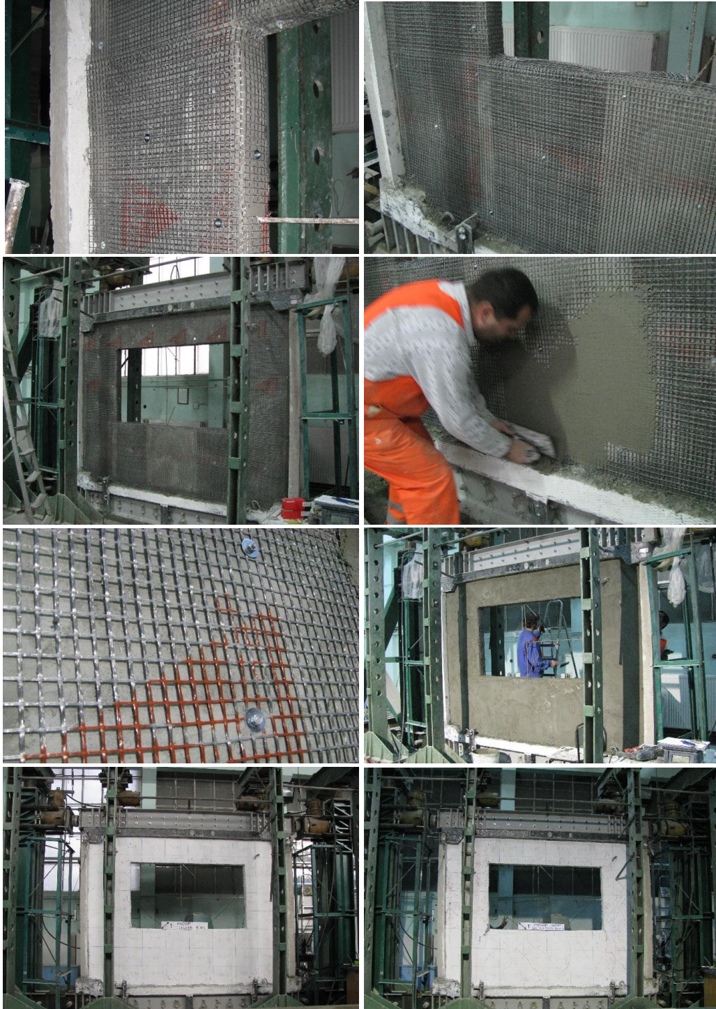
Figure 2.36 – FRP strengthening details
