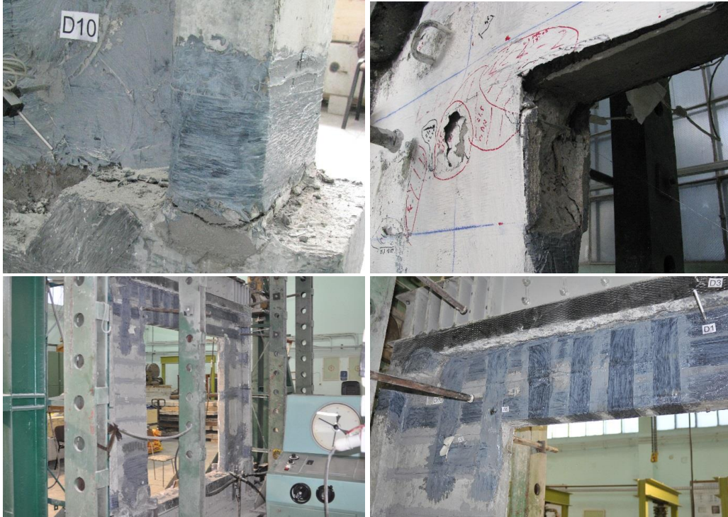
Figure 3.3 - Failure details of the PRCWP (9-E1/E3-R/T) specimen [109, 112, 118]
