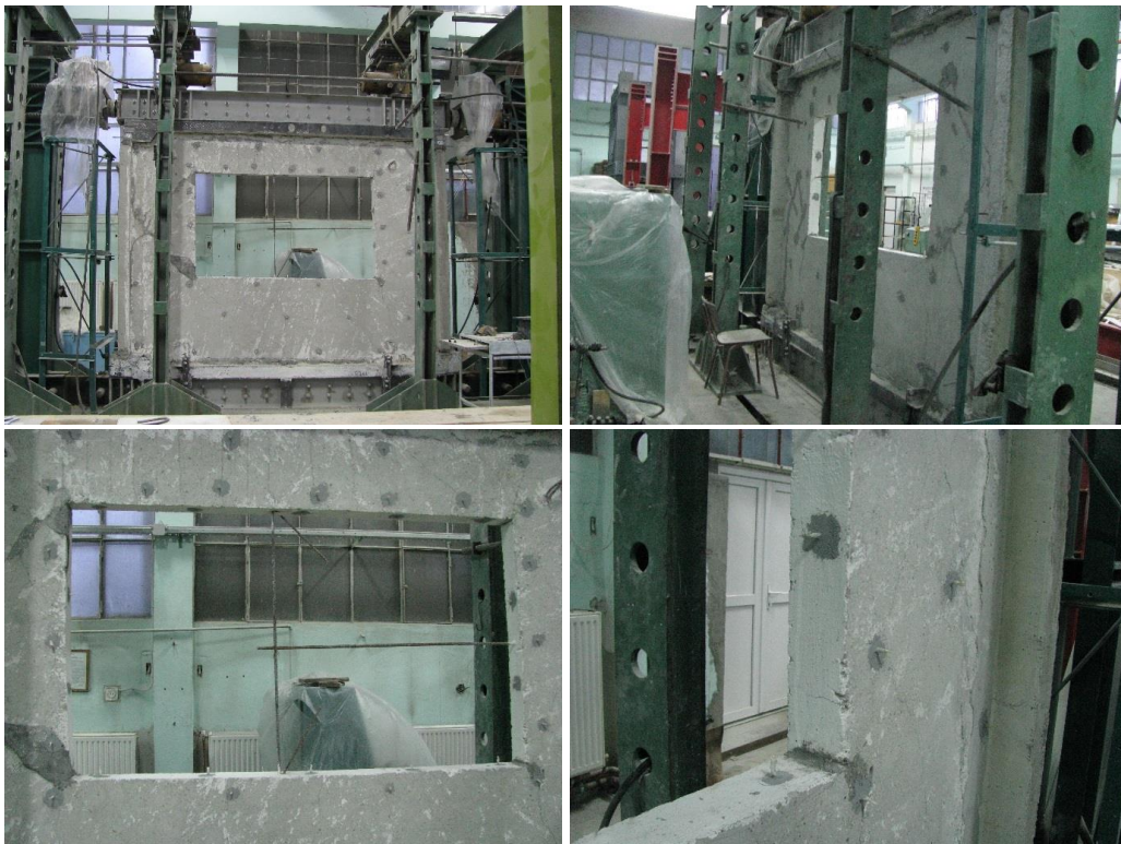
Figure 2.35 – FRP strengthening layout for PRCWP (10-L1/L3-T/R)
