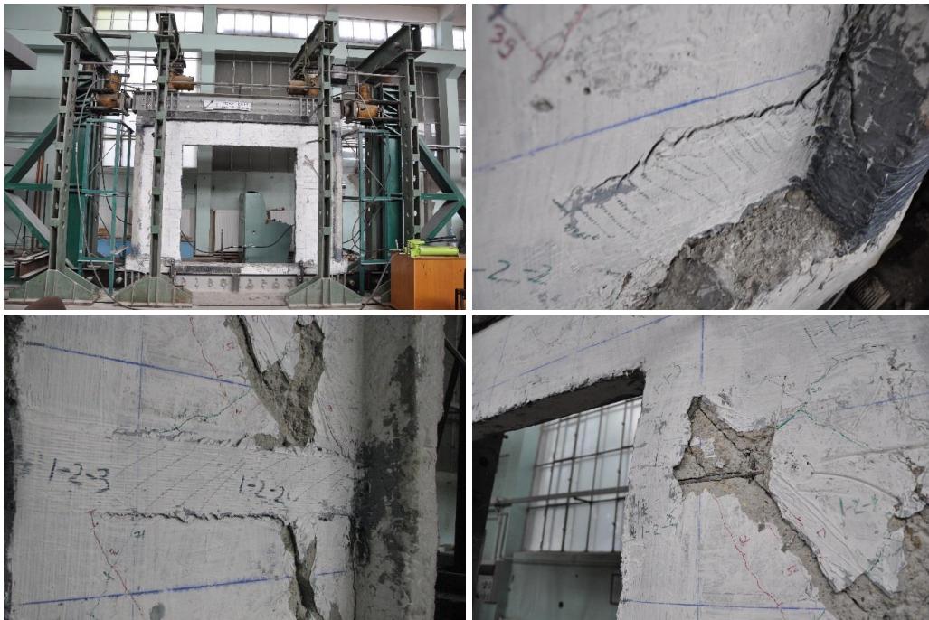
Figure 3.1 - Failure details of the PRCWP (7-E1-T/R) specimen [109-110, 112, 115]
