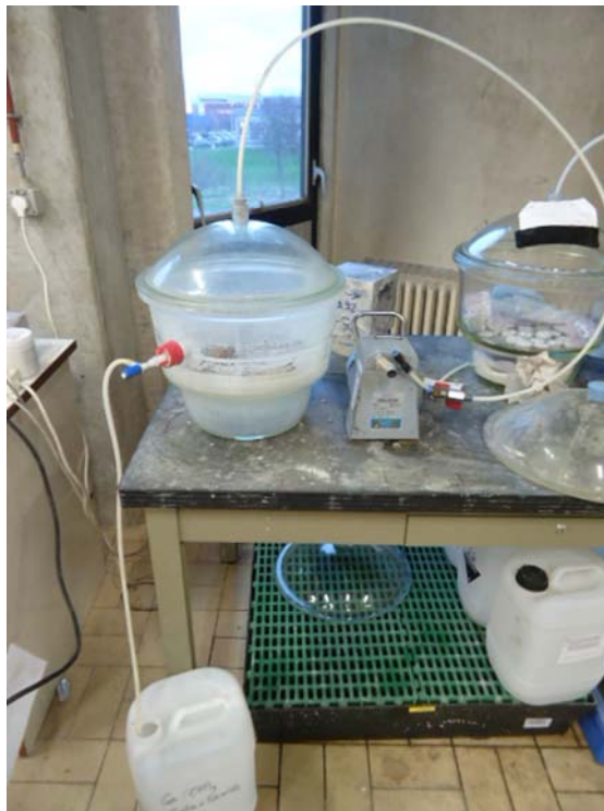
Figure 3.11. Equipment used for vacuum saturation
