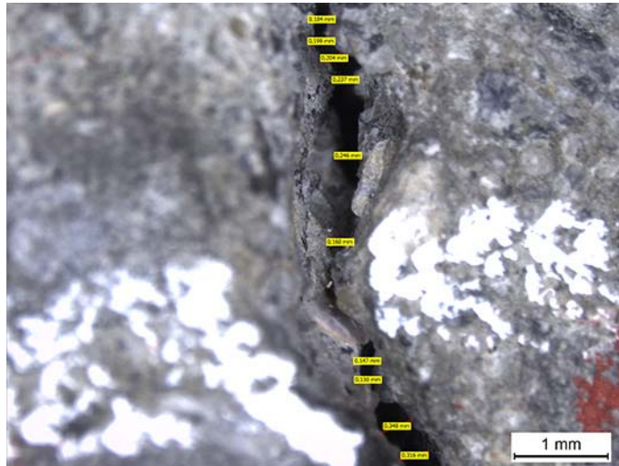
Figure 3.7. Measurement of crack width under the optical microscope
