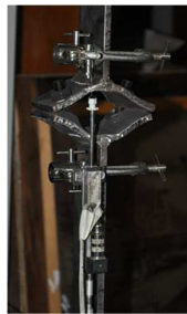
a) bolted T-stub preliminary tests
