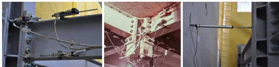
a) perimeteral column joint b) central column joint d) column horizontal deflection
