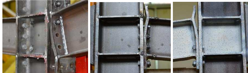
joint after the test: d) central column e) West column f) East column Figure 3.56. Experimental results for EP specimen [150]
