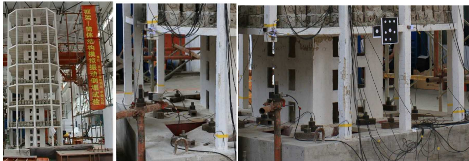
a) tested frame-core tube structure b) structure after static column removal c) removed column structure after shake-table test
