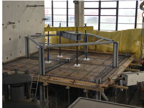
a) schematic representation b) illustration of the bottom reinforcement mesh [153] Figure 3.65. Reinforcement plan
