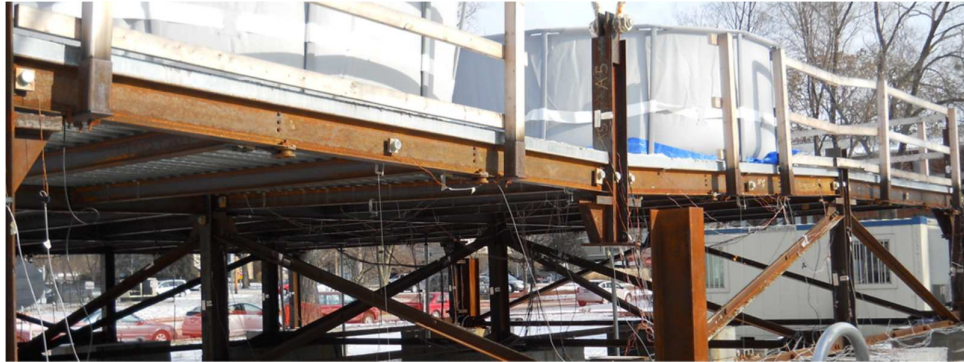
Figure 2.23 Edge column removal final equilibrium point [85]
