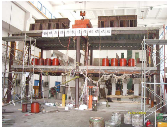
Figure 2.18 Experimental specimen subjected to sudden perimetral column loss [76]
