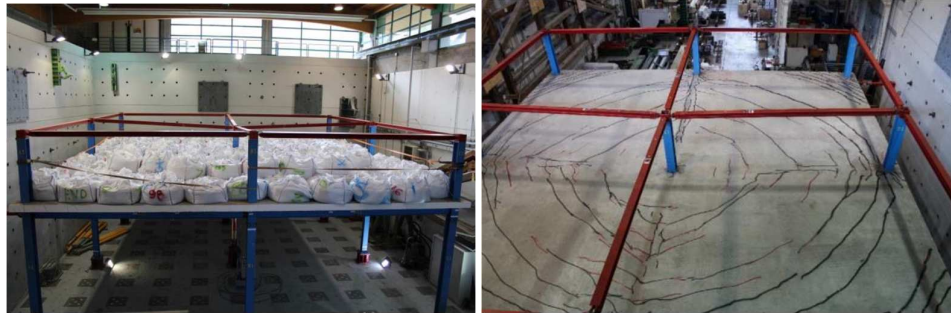
a) specimen at the end of the test b) Slab crack pattern Figure 2.19 Experimental results on symmetric 3D specimen [77]
