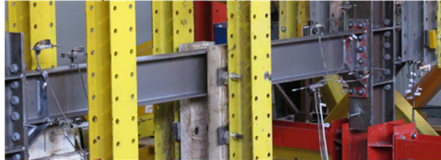
Figure 3.51. Overall view with position of the transducers on a specimen
