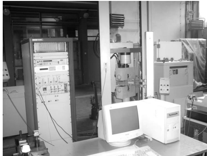
Fig. 5.4. Electro-mechanical test machine SCHENCK-TREBEL RM 100
