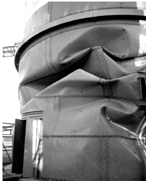
Fig.3.3. Cylindrical shell structure – buckling failure [3.5]
