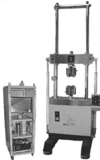
Fig.2.34. Fracture toughness testing machinery assembly
