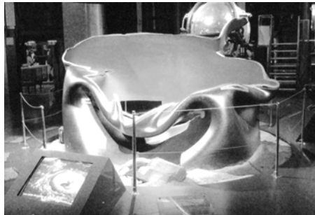
Fig. 1.10. Part of the bracing that failed during the accident (on display in the Norwegian Petroleum Museum)
