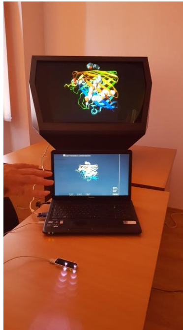
Figure 3.3. The IR lights of the LEAP Motion Controller
