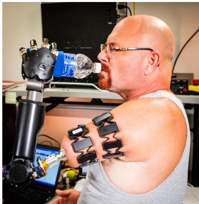
Figure 2.5. Two MYO armbands used to control a modular prosthetic limb (source: http://www.jhuapl.edu/newscenter/pressreleases/2016/images/20160112_8267_lg.jpg )
