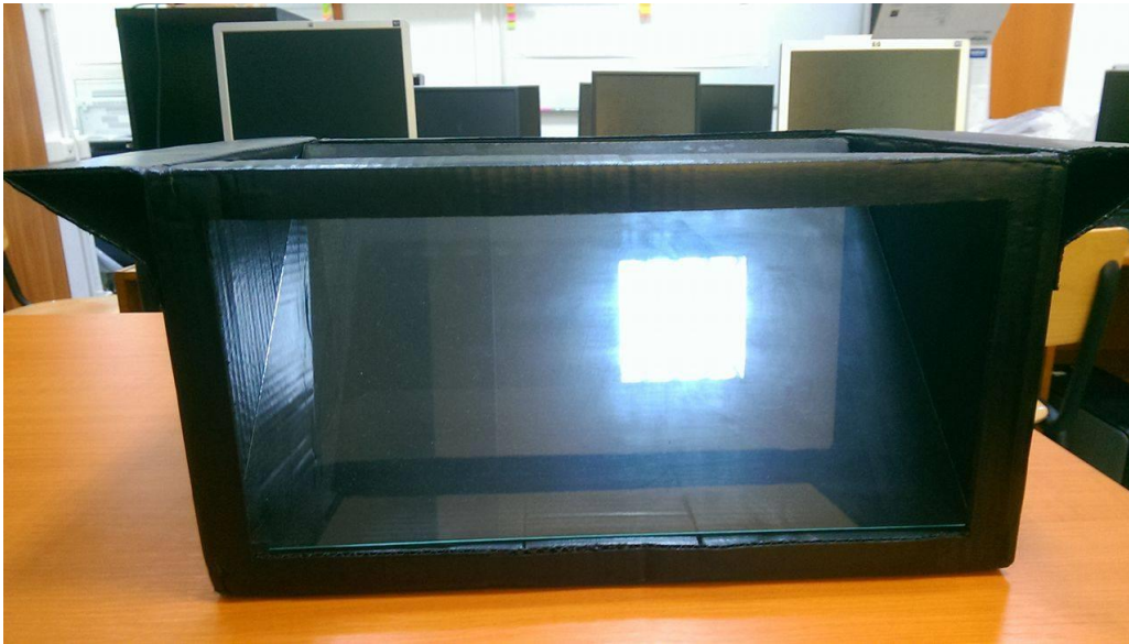
Figure 6.1. Custom-made pseudo-holographic 3D display
