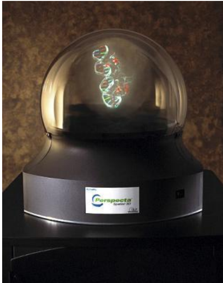
Figure 2.20. Volumetric display using a moving projection screen (source: http://i.stack.imgur.com/pO0M2.jpg )
