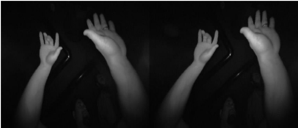
Figure 2.3. Objects illuminated by the infrared LEDs (source: http://blog.leapmotion.com/wp-content/uploads/2014/08/imageapi-hero.jpg )
