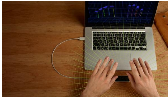
Figure 2.1. Leap Motion interaction space
