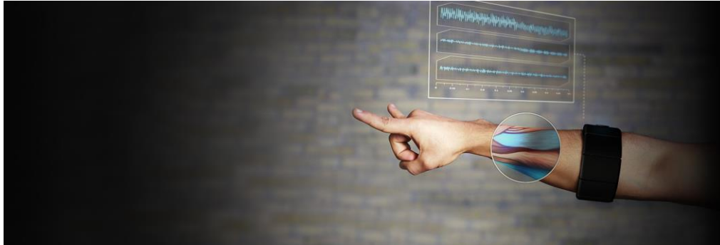
Figure 2.4. MYO detecting electrical activity in muscles (source: https://static.thalnic.com/img/arm_with_signal.jpg )
