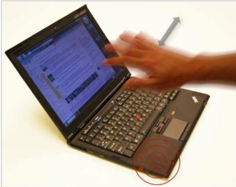
Figure 2.7. SoundWave in-air gesture sensing after [33]
