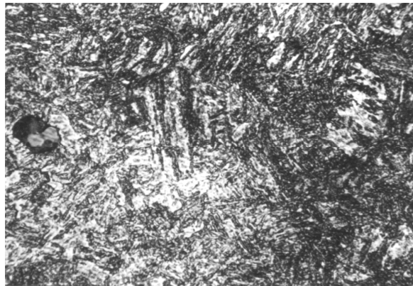
Fig.3.23. Proba MI , ZIT [ Atac Nital 2% , 100:1 ]
