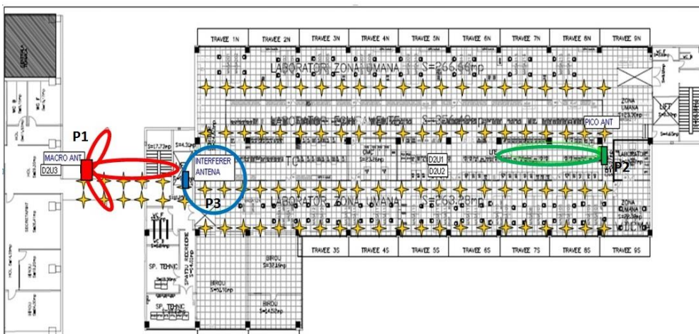
Figure 39: Building top view measurement points and cell locations. The macro cell is located at P1. The metro cell is located at P2 and interferer metro at P3
