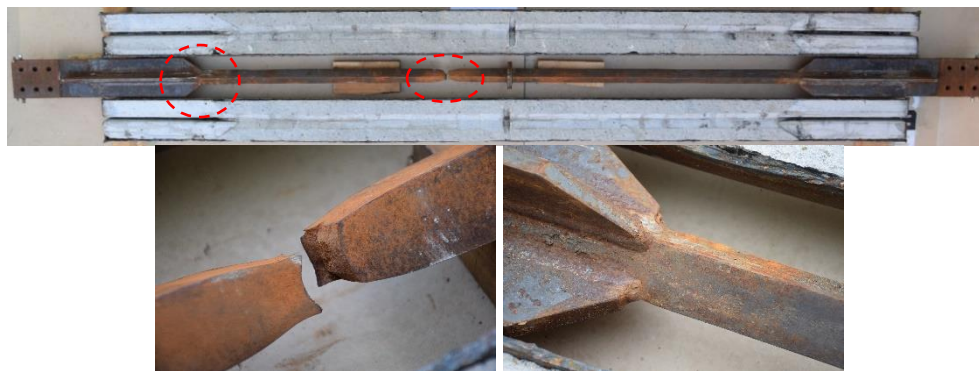
b) BRB type B: specimen CS73-2
