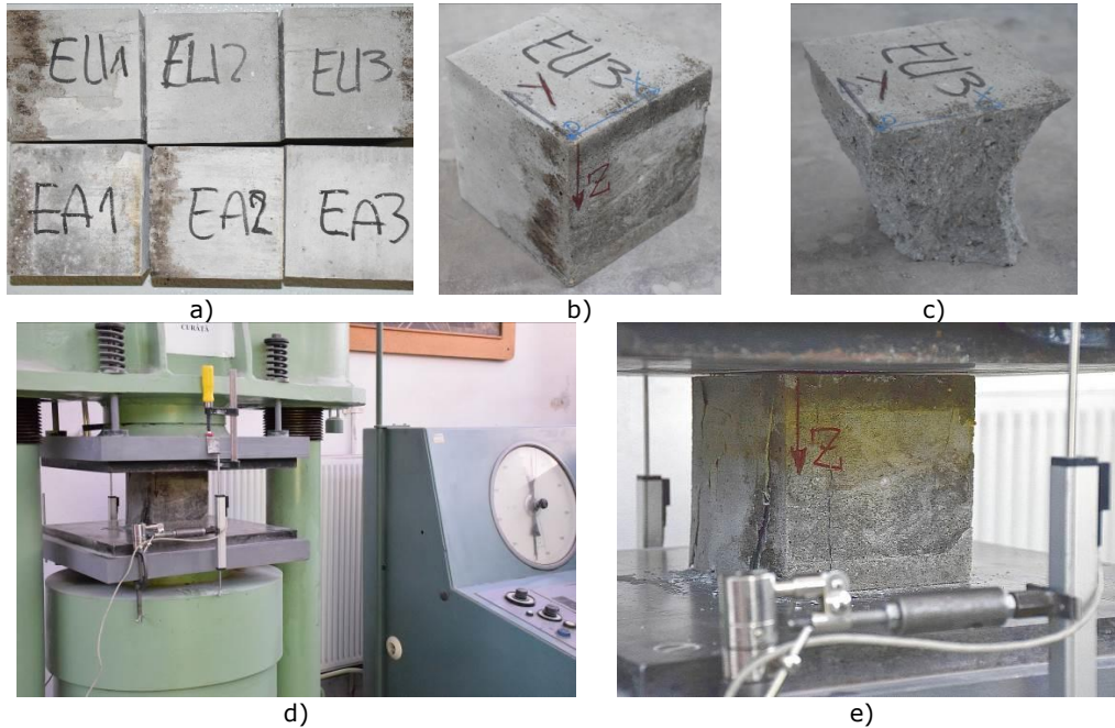
Fig. 4.11. Compression tests on concrete material: a) cubic specimens, b) perspective view of a specimen b) before and c) after test, d) testing machine, e) crack initiation
