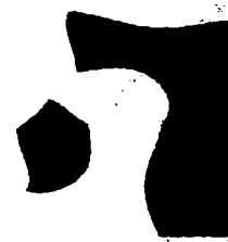
Fig.6 The space partition of the 4 MAQ output signals using a RBF equalizer
