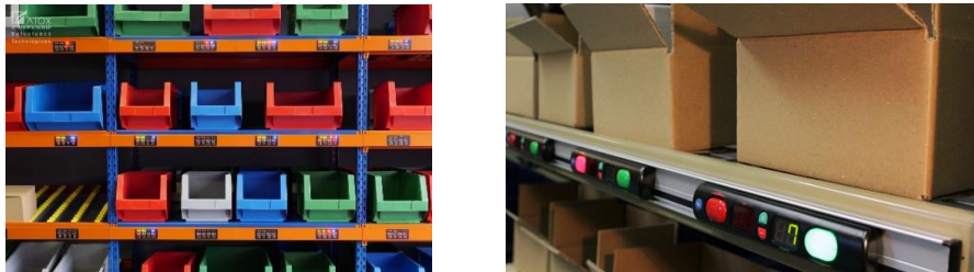
Figure 4.9. Pick to light system solutions (solutions from Atoxgrupe 42 ; Lightning Pick 43 cite by (Mocan and Draghici, 2019a))
