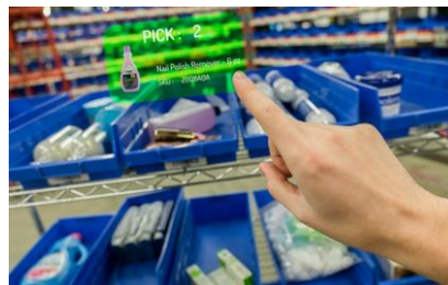
Figure 4.10. Bastian solutions AR picking technology 44 (Mocan and Draghici, 2019a)
