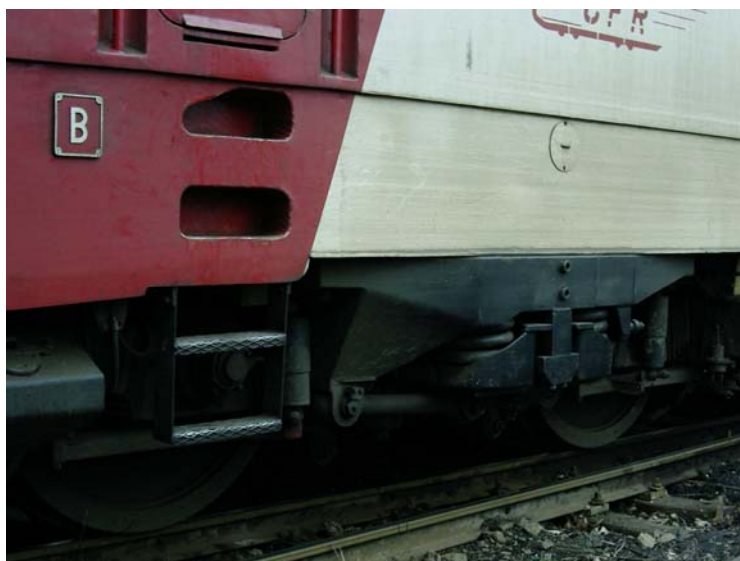
Fig. 1-21. Suspensia locomotivei electrice de 3600 kW
