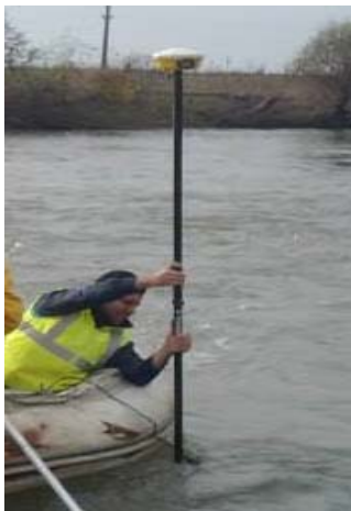
Figure 11. Positioning the active transducer over the water surface
