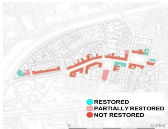
Figure 3.24. The conservation state for the investigated buildings in Fabric district [174]
