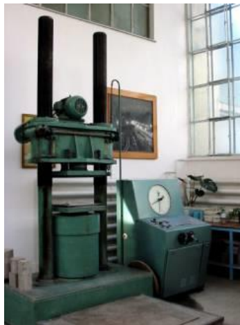
Figure 3.61. Hydraulic press used in the experimental tests on burnt clay brick extracted from some of the historical investigated buildings in Timisoara [211]
