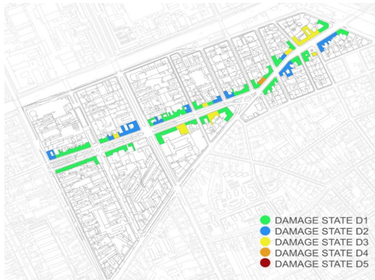
Figure 3.133. Seismic vulnerability map for Iosefin historical district, for first 10 parameters based on proposed adapted methodology [174]
