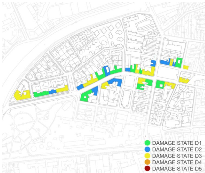
Figure 3.134. Seismic vulnerability map for Fabric historical district, for first 10 parameters based on proposed adapted methodology [174]
