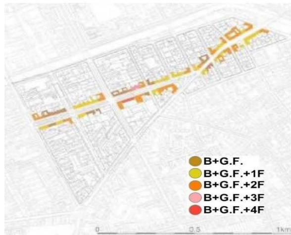
Figure 3.17. Height regime for the investigated historical masonry buildings in Iosefin district [174]
