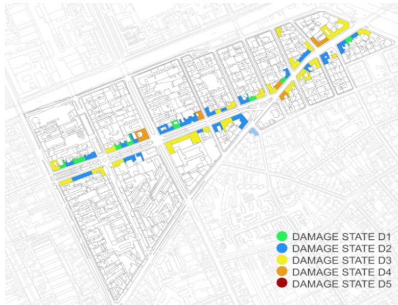
Figure 3.143. Seismic vulnerability map for Iosefin historical district, for all 15 parameters based on proposed adapted methodology [174]
