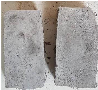
Figure 3.63. Some of the tested burnt clay brick after the application of a lime topping [211]
