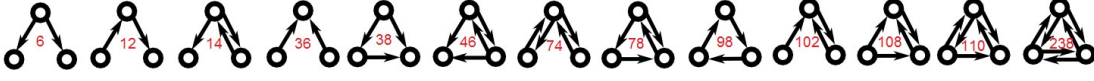
Figure 2.8 All existing motifs of size 3 in a directed graph. The code of each motif corresponds to the decimal value of its serialized adjacency matrix [193].
