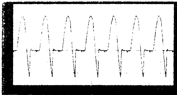
Fig 9 The dropping voltage in case of resistive-inductive load for one phase rectifier
