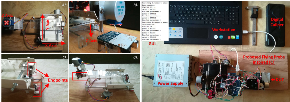
Fig. 6.1. Left: FPICT Mechanical Structure with Axis Array (a, b) and MELS Placement (c, d). Right: Complete experimental setup for the proposed FPICT.
