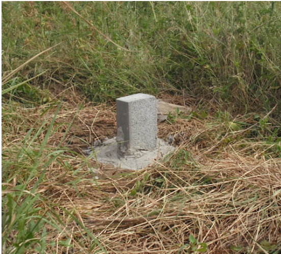
Figure 7. Marking and signaling of topographic points (S1, S2) concrete landmark
