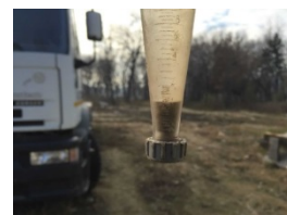
Figure 8. Sedimentation cone-Value 1.00 ml.-1.80 gr
