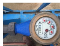
Figure 6. Flowmeter with the maximum accuracy of 0.0001 m 3
