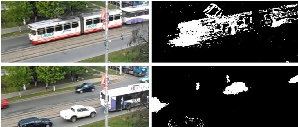
Figure 32 - Left original frames , right the foreground masks generated by the MOG algorithm
