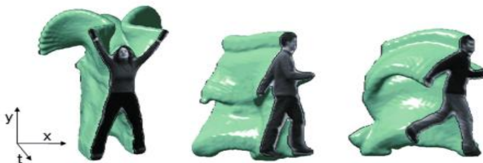
Figure 11 - Illustration of space time shapes for three types of actions, namely for jumping-jack, walking and running [28]
