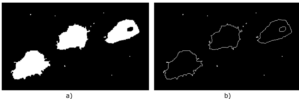
Figure 37 - a) Foreground mask after correction; b) The contours of the vehicles detected by the algorithm of Suzuki and Abe
