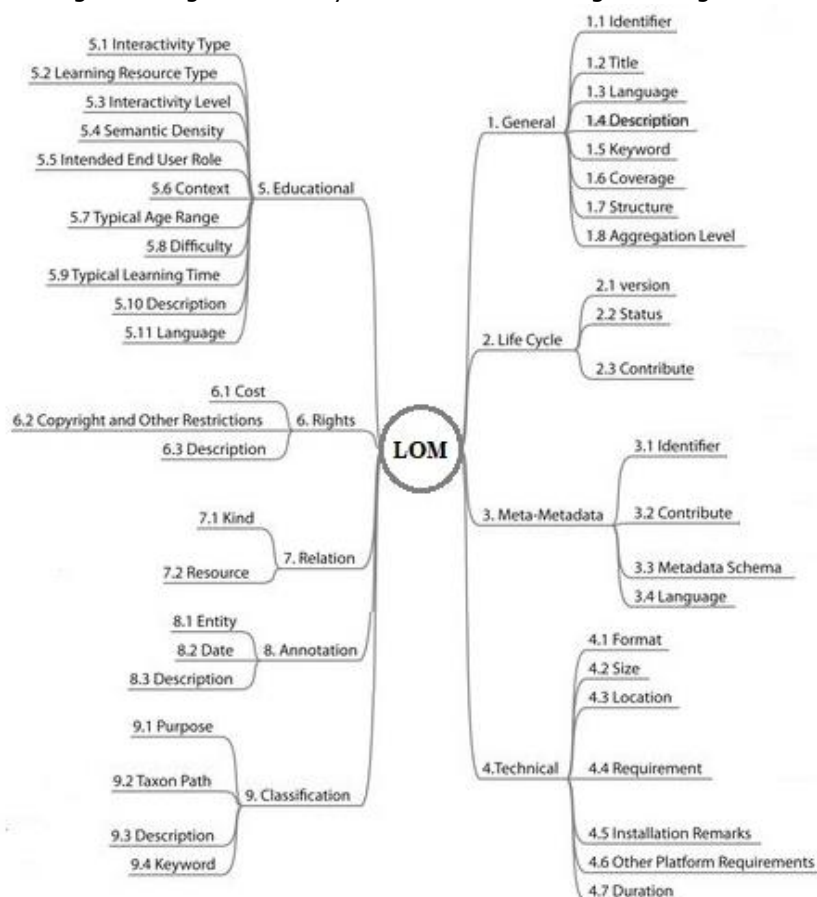
Fig.2.1. The hierarchy of elements in the LOM data model
